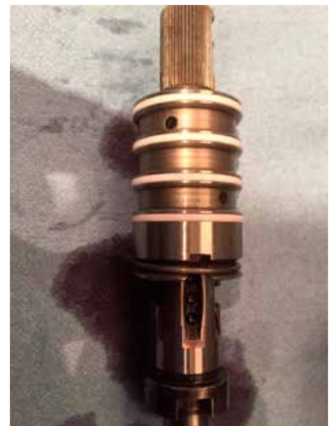
Align the two holes in the bobbin with the three slots in the input shaft.
