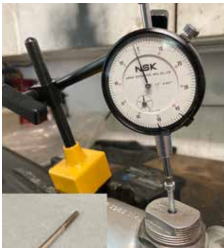
The plunger adjustment. Inset is the bolt I use
