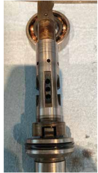
Before inserting the roll pins, ensure the lug is centred
