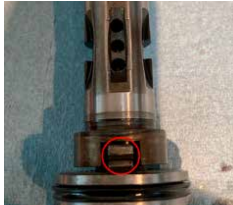
Mark the lug (circled) that aligns with the three slots
