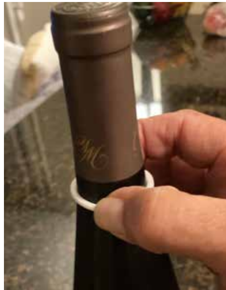
Stretching the heated PTFE seals over a wine bottle
