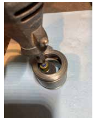
Cleaning out the main seal grooves
