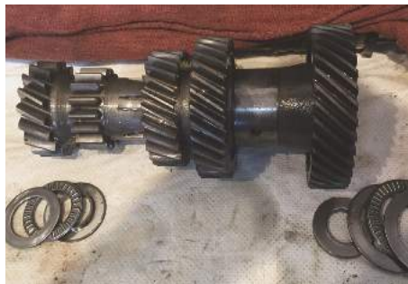
Stag layshaft with roller thrusts. The shaft is thicker at one end
