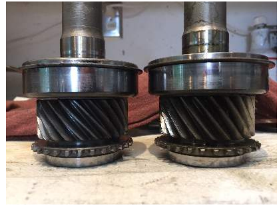
Helix - note the different gear helix angles in these input shafts. Left is the earlier helix angle
