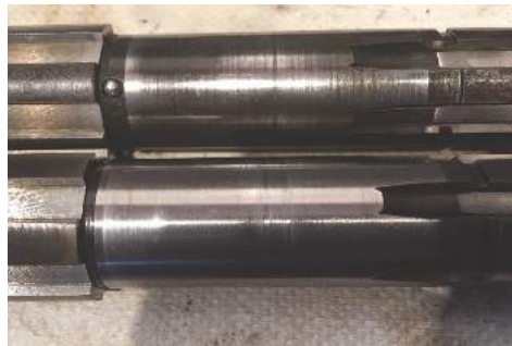
Two types of mainshaft - the one at the top has the ball bearing for the tophat type
