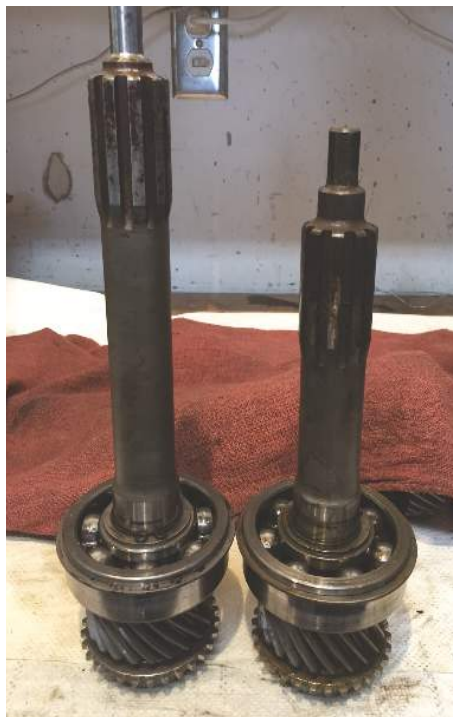
Input shafts - the left shaft is an early type Stag input shaft; the right a late TR6. Note the extra length of the Stag shaft
