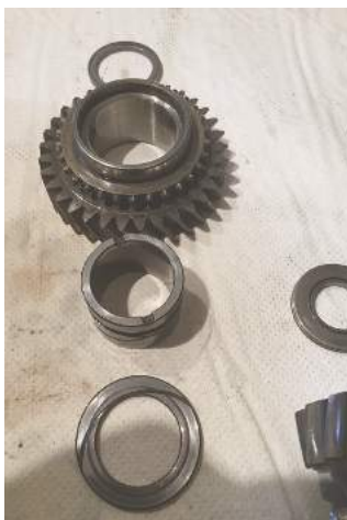
Two-piece steel 2nd gear. The bushing and thinner-type spacer is from an early Stag gearbox
