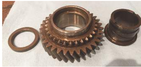
The "Tophat" steel 2nd gear, its bushing and thicker spacer from the later Stag gearbox
