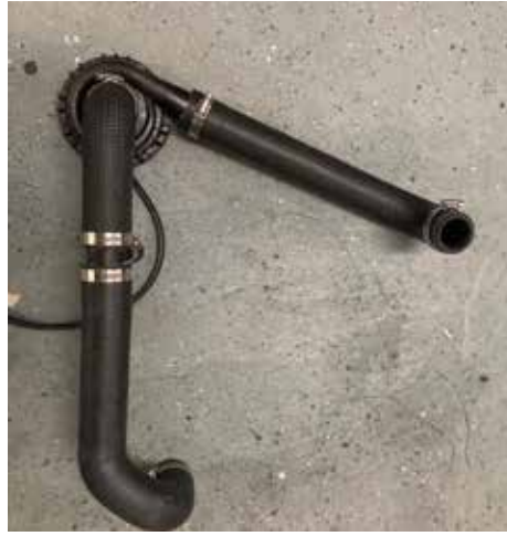
EWP pump and hoses
