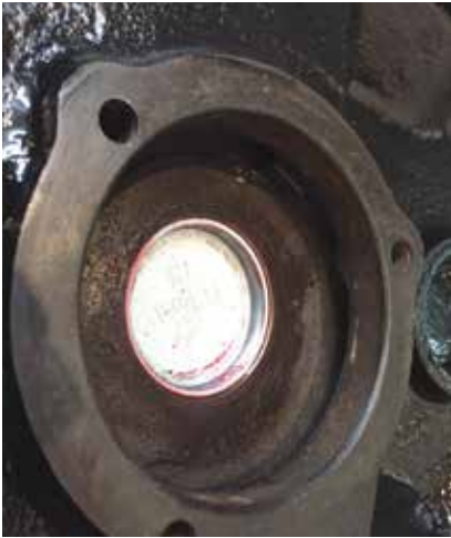
Original water pump plugged off
