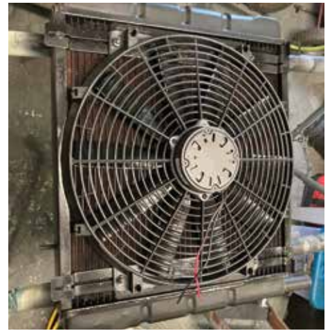
A 16" electric pusher fan is controlled through the Davies Craig controller box
