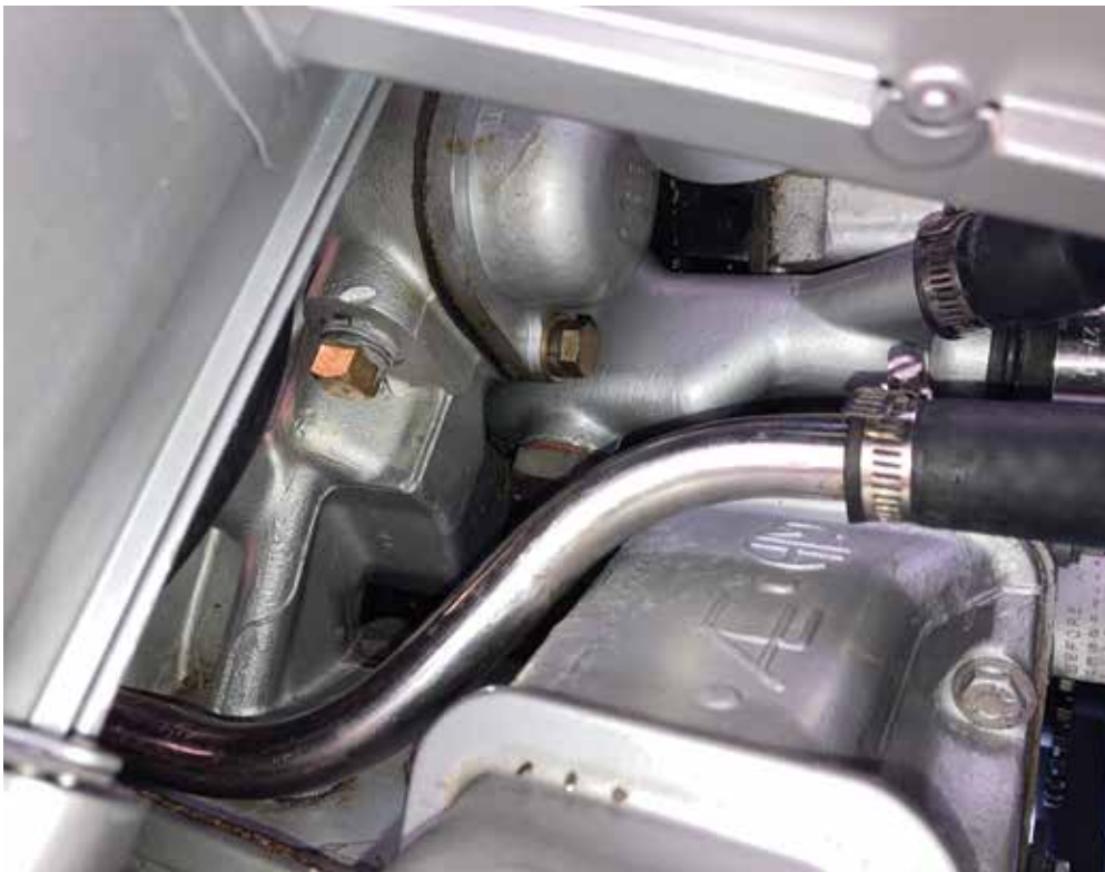
The thermostat was removed and the by-pass hose connection from the inlet manifold was plugged, as well as the by-pass/heater inlet to the pump cover
